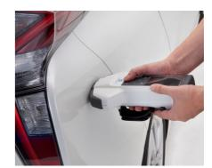
The compact body (with hand strap) can be stably held with one or two hands. Moreover, it is loaded with features ideal for measuring vehicle exteriors such as a rubber cover around the measurement aperture to safeguard measurement subjects against scratching and Bluetooth® support (option) for sending measurement data to remote devices over wireless connections.
