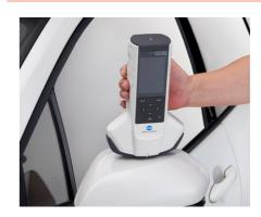
The viewing beam is 6 mm in diameter, so small surfaces that were hard to measure with earlier models can be stably measured.
